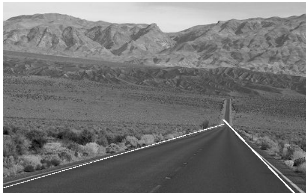
Figure 6.16 Line fitting approximation to the previous result.
