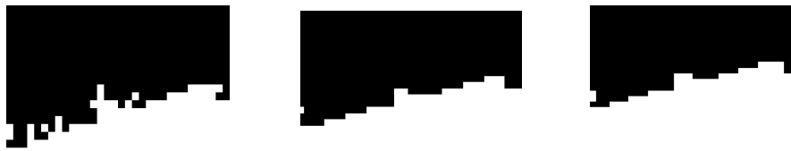
Figure 3.8 left one is the intermediate result for road image, middle erosion image, and right one dilated of the eroded image with structuring element 17.
