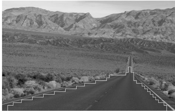
Figure 6.15 Extractions of road borders obtained by three dimensional texture space.
