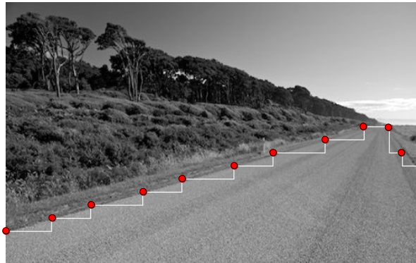
Figure 5.34 Leftmost points used to fit line on staircase.
