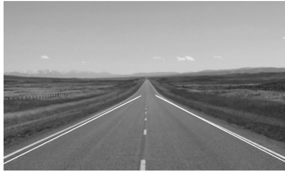
Figure 6.4 Extraction, where the lane borders are visible and final borders fitting.
