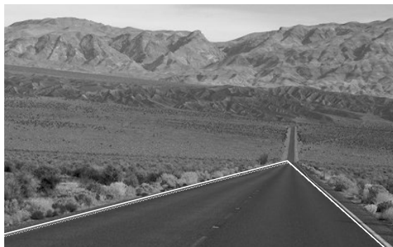
Figure 6.2 Extracted borders before slope point.
