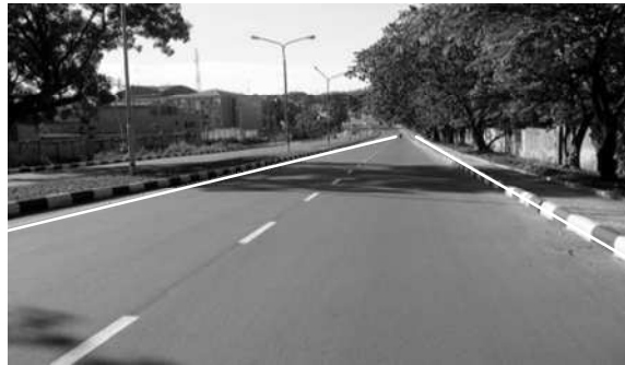
Figure 6.14 Final results obtained after border fitting into 2D classification.
