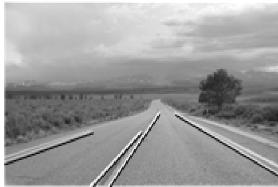
Figure 6.6 The Extracted borders are intensified in black.
