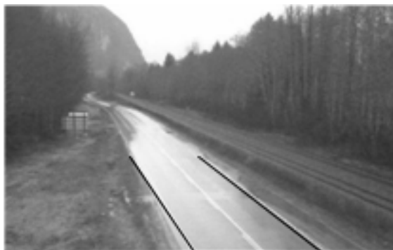
Figure 6.8 Extracted borders are intensified in black.
