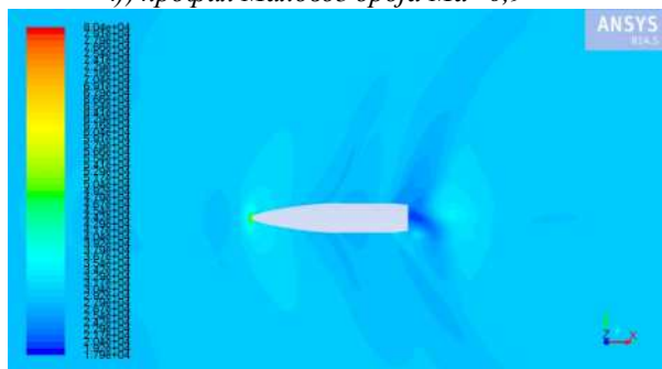
Contours of Static Pressure (pascal) (Time=1.0000e-03) Feb 27, 2014 ANSYS Fluent 14.5 (3d, dp, dbns imp, LES, transient)
