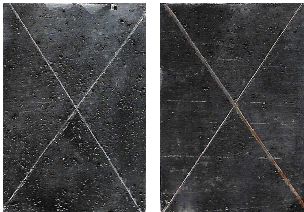
Fig. 4.40. Images of the mild steel samples with base coating + 5 wt.% ESEC before (left) and after 10 days (right) of exposition in wet chamber.
