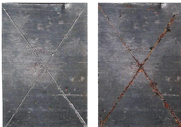
Fig. 4.37. Images of the mild steel samples with base coating before (left) and after 10 days (right) of exposition in wet chamber.
