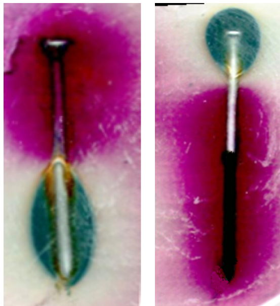
Fig. 4.17. Ferroxyl indicator test of an unprotected (left) and a PANI-protected nail (right) after 10 h.
