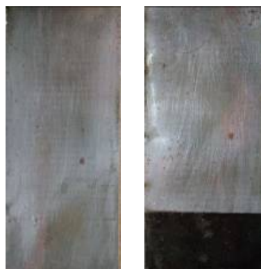
Fig. 4.12. Images of mild steel (left) and mild steel partially covered with polyaniline (right) after a 60-day exposure to dry Sahara sand..
