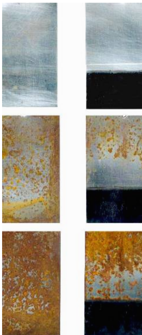
Fig. 4.14. Images of the mild steel samples after 1 (top), 15 (middle) and 45 (bottom) days exposed to atmospheric corrosion in Belgrade downtown. Left: bare mild steel, right: mild steel-PANI-benzoates.
