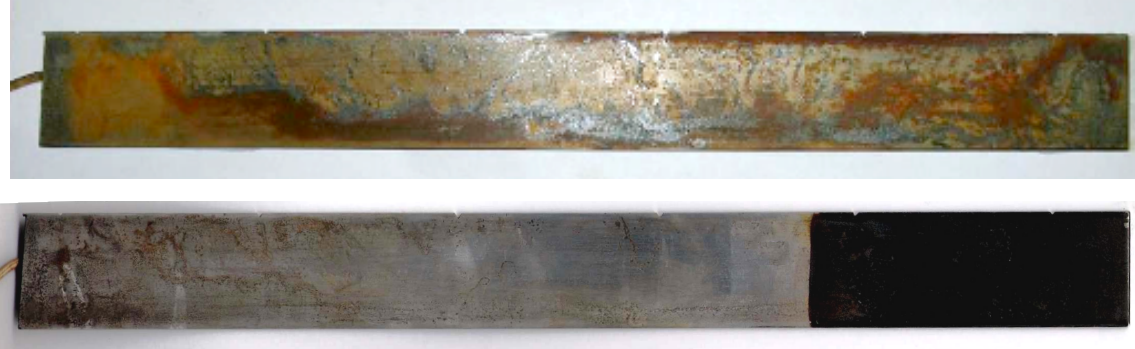
Fig. 4.11. Comparison of the images of bare mild steel and mild steel with partial PANI-benzoate coatings after a ten-hour exposure to 3% NaCl at the corrosion potential.
