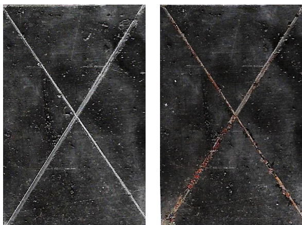
Fig. 4.41. Images of the mild steel samples with base coating + 5 wt.% EBEC before (left) and after 10 days (right) of exposition in wet chamber.
