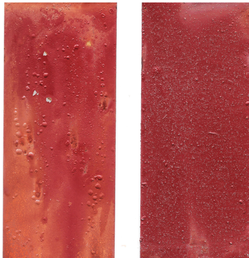
Fig 4.59. Images of the samples after 200 h of corrosion in 3% NaCl. left: TESSAROL-Helios primer for iron paint; right: TESSAROL-Helios primer for iron + 5 wt% ESC (based on dry paint).
