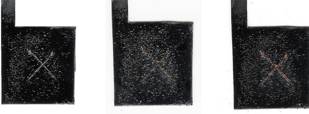
Fig. 4.58. Images of mild steel covered with 30 \mu\text{m} base coatings + 5 wt.% of polyaniline ESC before immersion (left), after immersion for 24 h (middle) and 80 h (right) in 3% NaCl.
