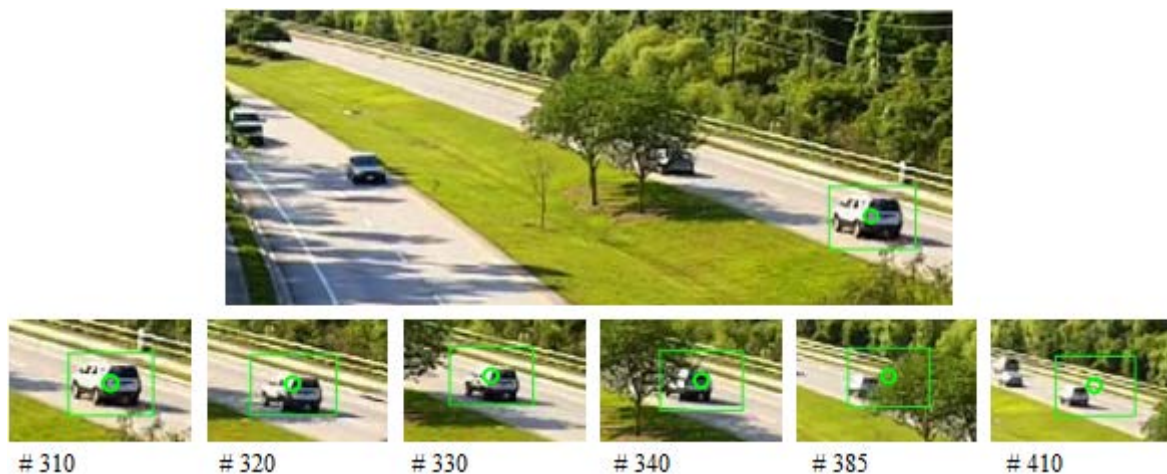
Fig.5.8 Selected real scenario for checking the parameters on the proposed tracking algorithm
