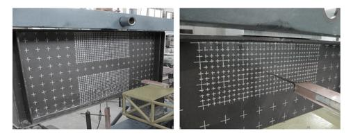
Figure 3.5: Measuring initial geometric web panel imperfections using a rectangular grid size of 21x11 points.
