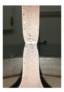
Figure A.2: Typical coupon specimen failure.
