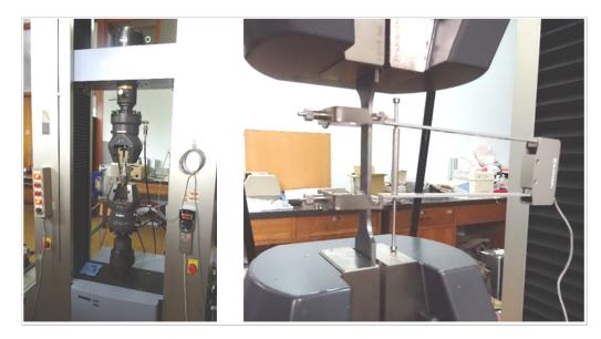
Figure A.1: Universal Testing Machine Shimadzu AG-Xplus and extensometer with an initial length of 50 mm.
