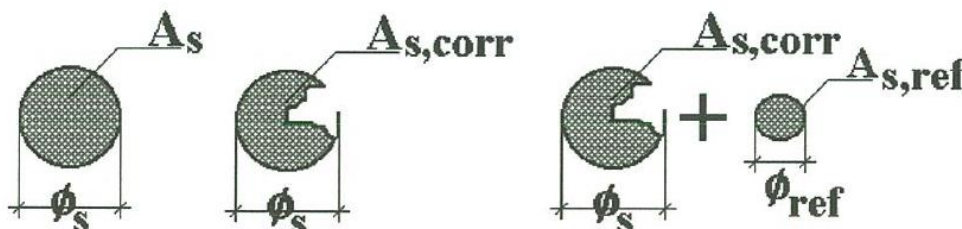
Figure (VIII-11): Calculation of lacking reinforcement area
