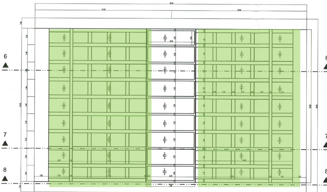
Figure VI-13. Arch slab view from bottom side and location of cantilever arch slabs
