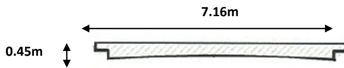
Figure VI-72. Dimensions of simple beam slab in cross section
