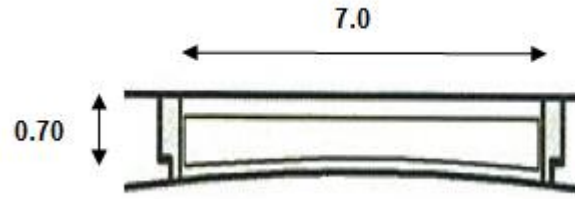
Figure VI-18. Dimensions of simple supported beam slab in cross section
