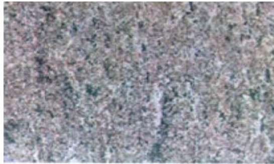
Figure (VIII-7): Requested visual cleanliness of bars – preparation grades Sa 2
