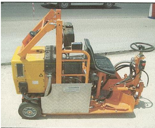
Figure (VIII-39) Special machine for open and clean cracks
