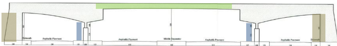
Figure VI-94. Disposition of exterior (blue), interior walls of bridge (grey) and deck ceiling slab
