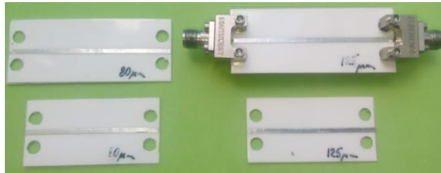
Figure 6.3 The layouts of the microstrip line with SMA connectors used for permittivity characterization [13]
