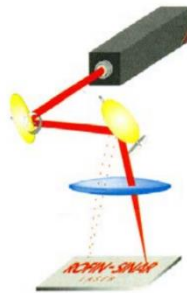
Figure 4.10 Manipulation of the laser beam according to the PC signal inside the marker head
