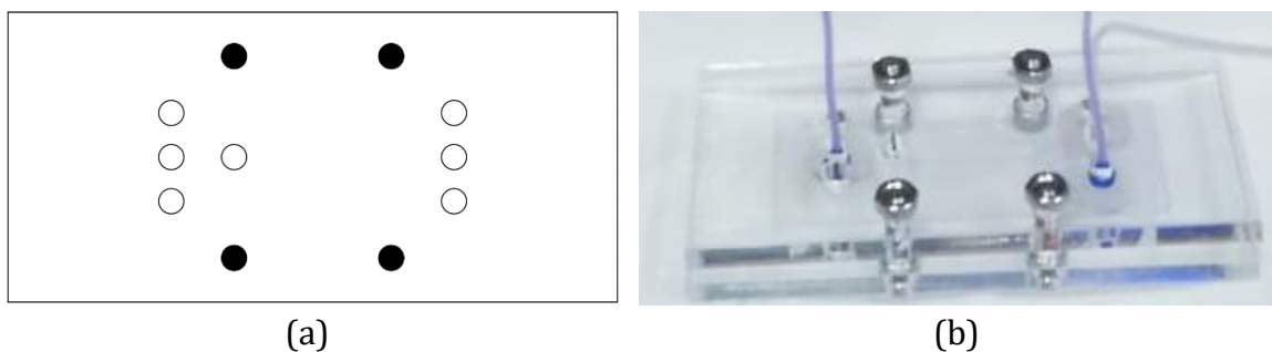
Figure 7.2 Holder for PVC and SAVA fabricated microfluidic chips (a) design, (b) picture
