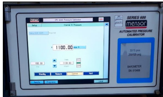
Figure 5.16 Typical operation screen
