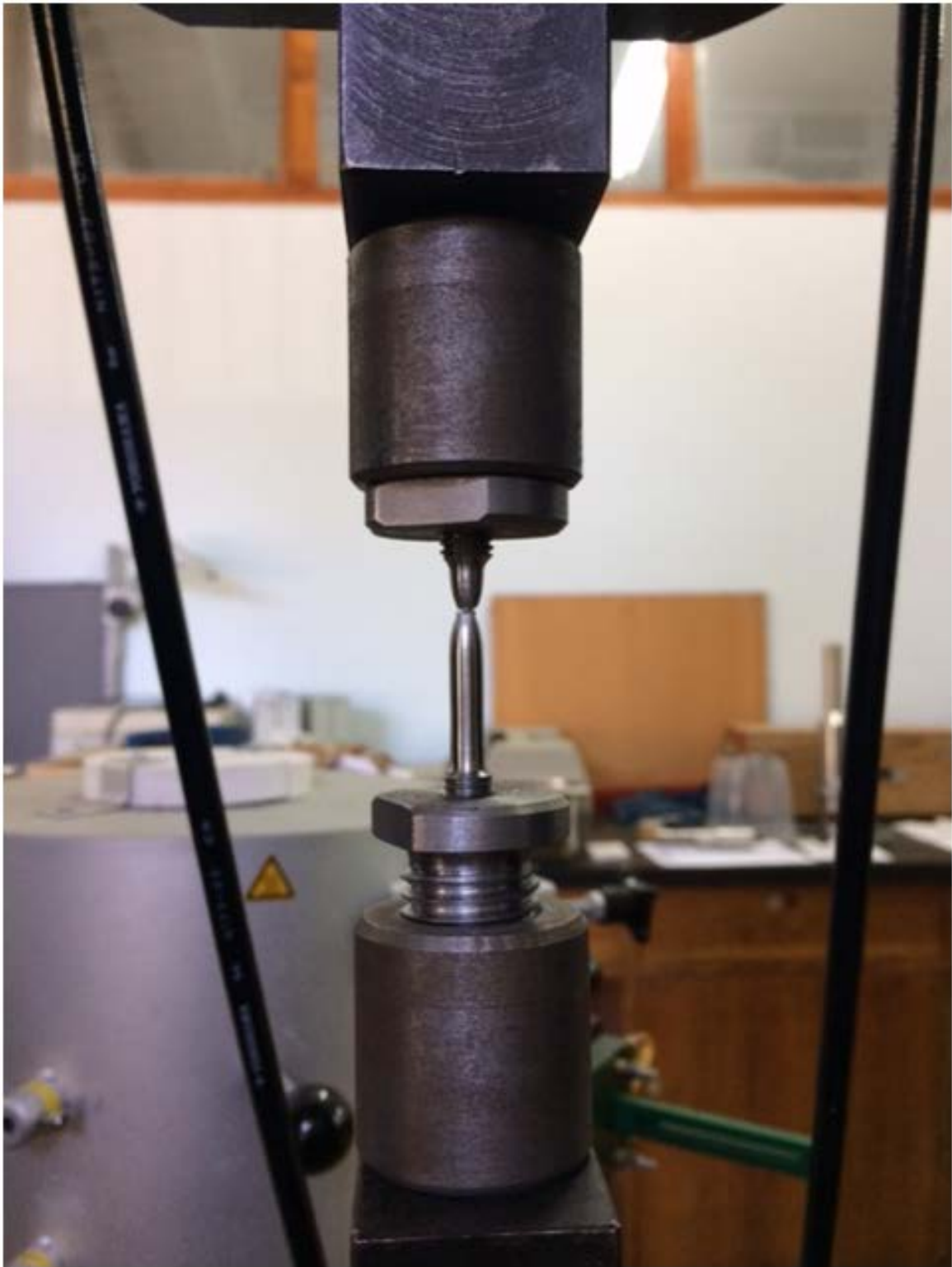
Figure 3.2. The end of tensile test with broken specimen positioned in the testing jig
