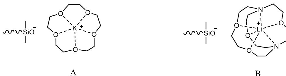
Figure 2.2. Separation of metal cations from silanolate anions by the use of crown ethers (A) and cryptates (B).
