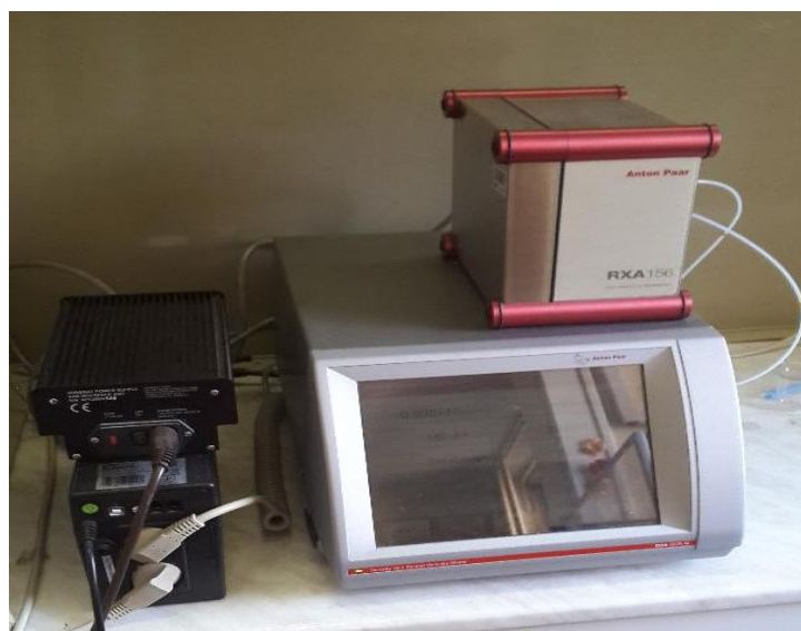
Figure 3.13 RXA 156 Refractometer connected to DSA 5000 M Density and Sound Speed Measurement Device.
