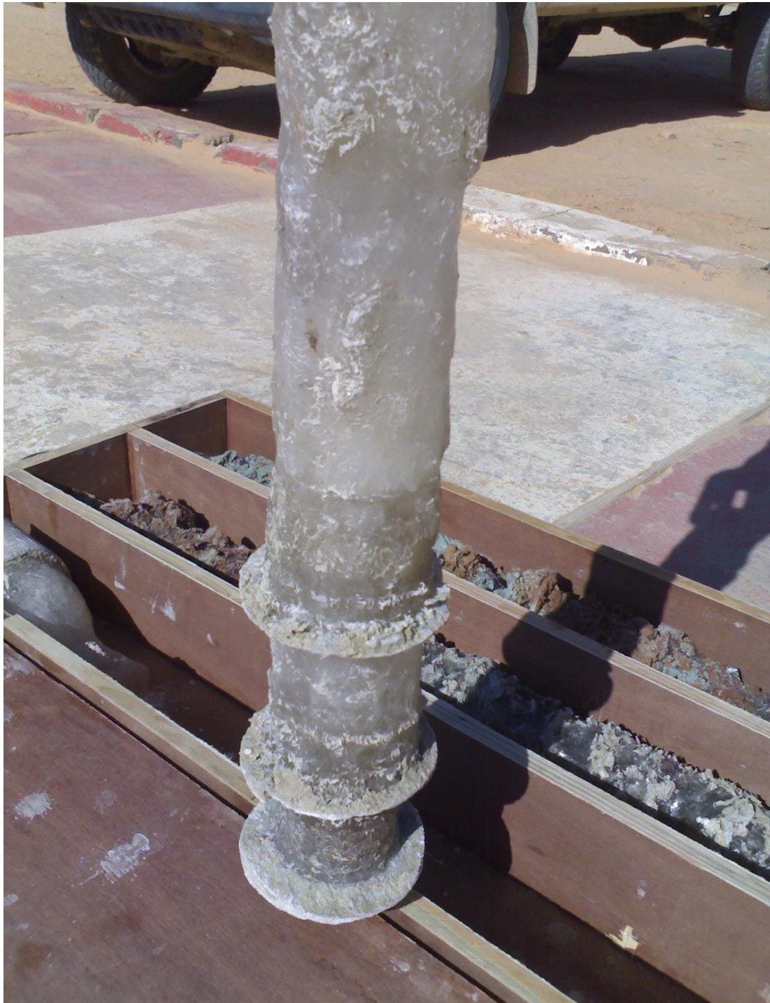
Figure (62 C):- Cylindrical core sample of Ain Tobi Member/ Sidi Assid composition at a depth of 377 meters in the well number (PZ-Zk)
