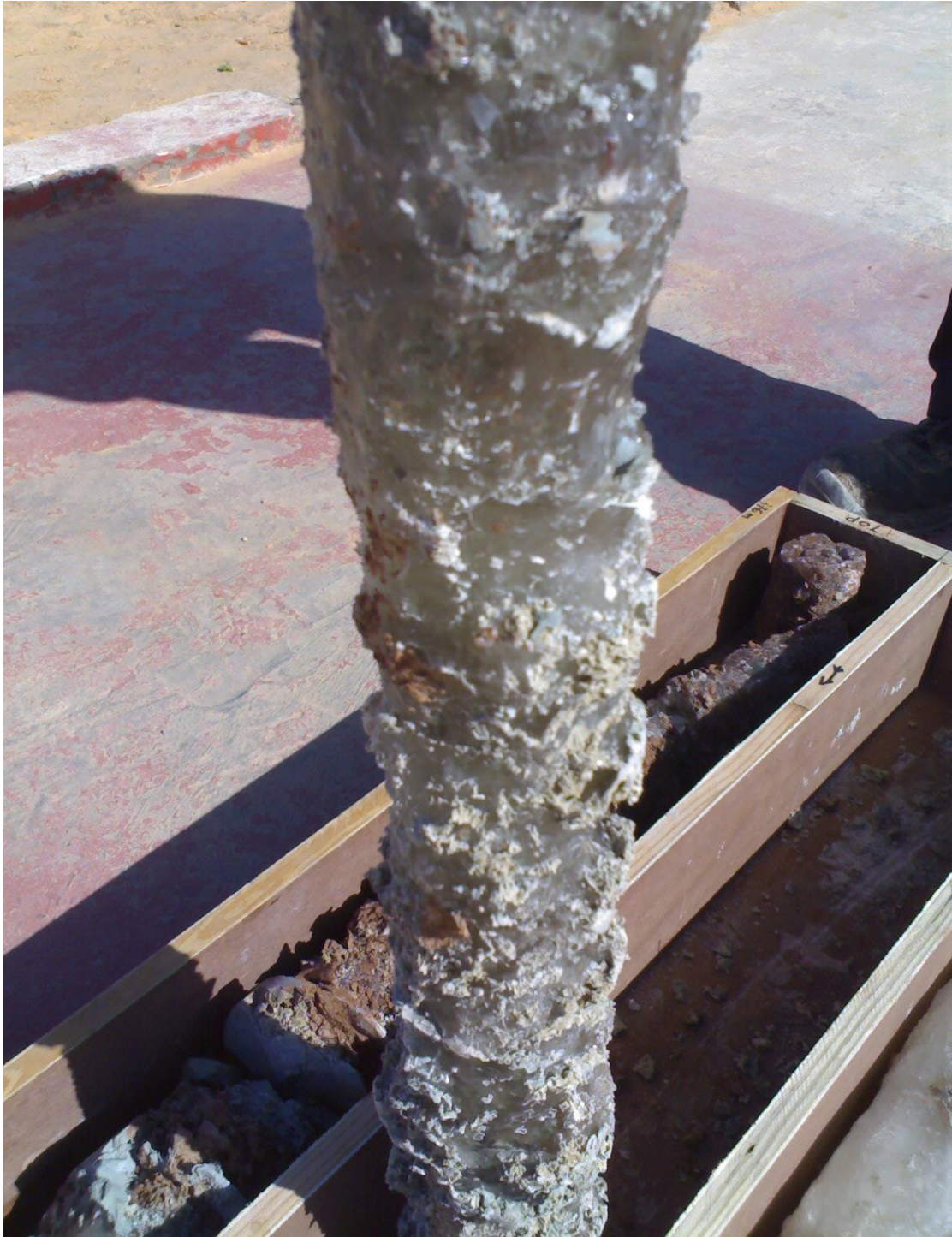
Figure (62 B):- Cylindrical core sample of Ain Tobi Member/ Sidi Assaid composition at a deep of 377 meters in the well number (PZ-Zk)
