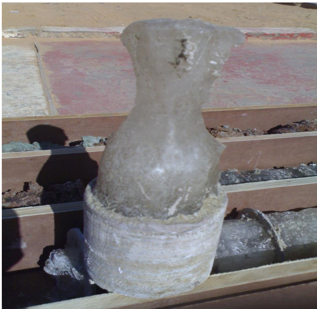
Figure (62 A):- Cylindrical core sample of Ain Tobi Member Sidi Assaid composition at a deep of 378 meters in the well (Pz-7k)
