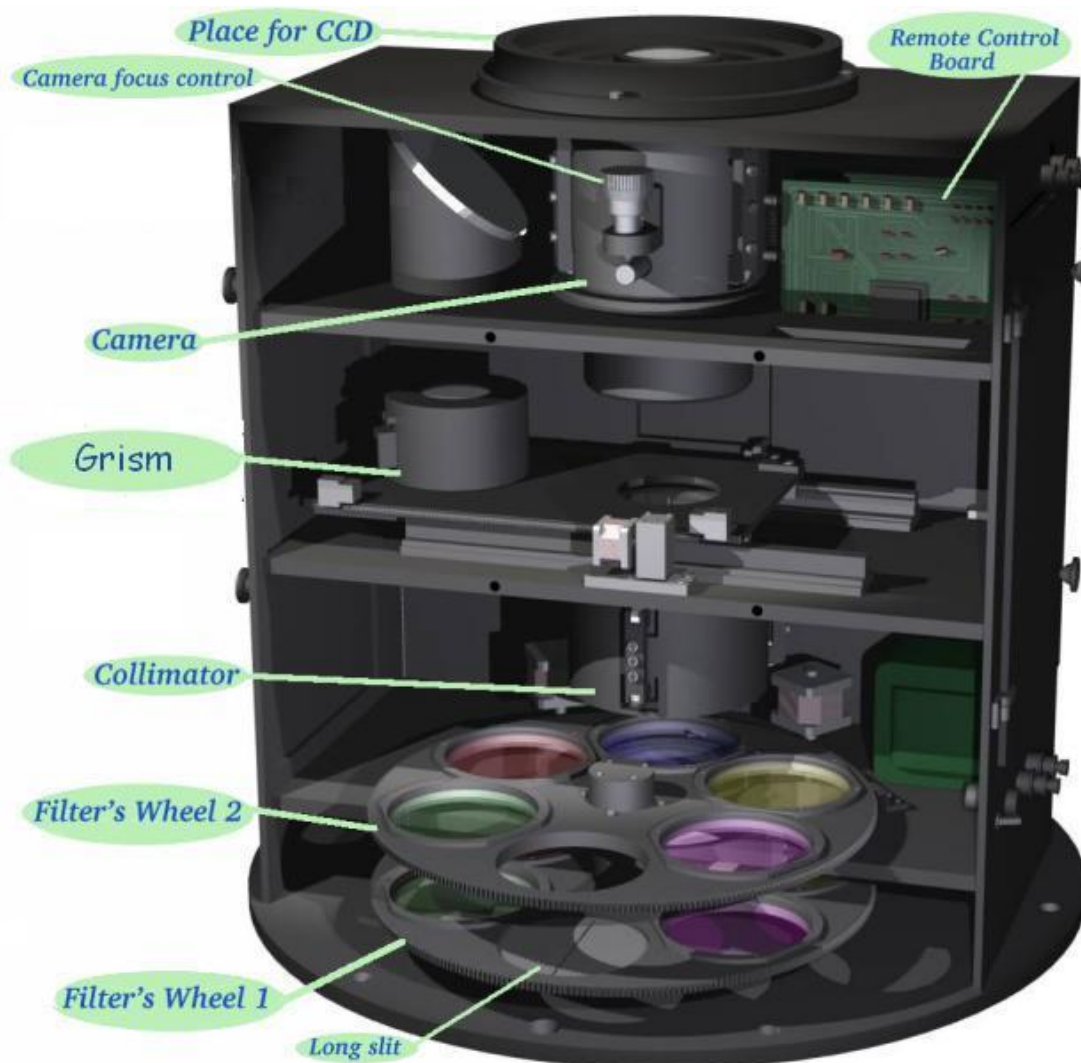
Figure 6.6: Upper panel: the optical scheme of the polarimetric mode of the focal reducer SCORPIO: 1–slit; 2–the phase plate; 3–the collimator, 4–the Wollaston prism; 5–the grism; 6–the spectrograph camera; 7–the entrance window of the CCD (charged coupled device) cryostat. Credits: Afanasiev & Amirkhanyan (2012). Bottom: a real picture of SCORPIO with all its optical elements marked in the figure. Credits: SAO RAS gallery https://www.sao.ru/hq/lsvfo/devices/scorpio/scorpio.html .
