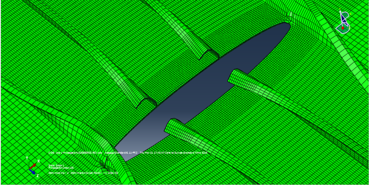
Figure 5.26 Crack after 138 steps of propagation.
