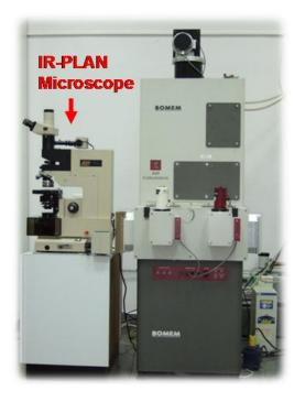
Figure 34. BOMEM DA-8 FIR spectrometer.
