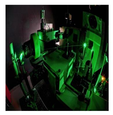
Figure 33. Raman spectrometer Jobin-Yvon T64000.
