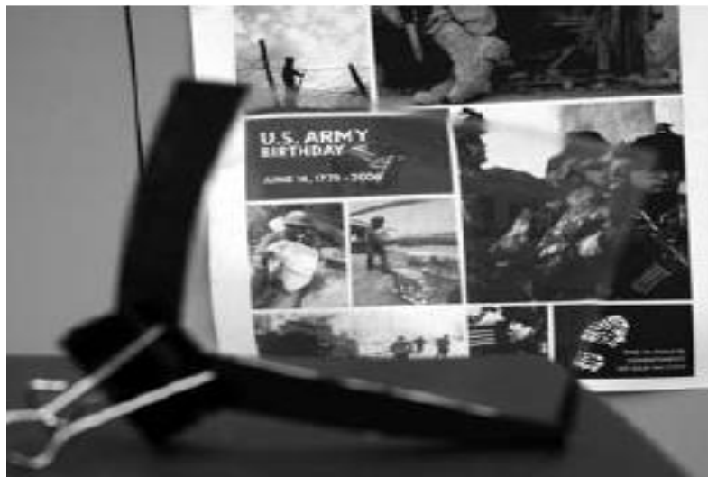
Figure 25. Translucent PMMA electrospun PVB-fiber composite [188]
