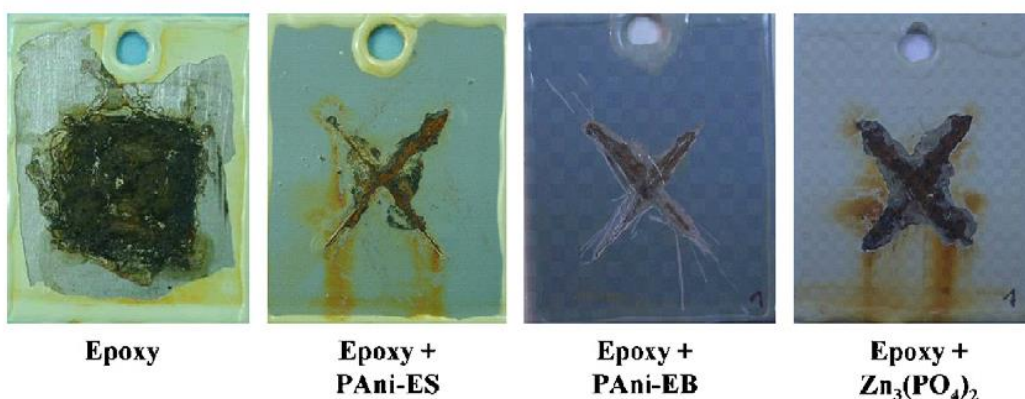
Figure 2.14. Scrapped test panels of epoxy, epoxy + PAni-ES, epoxy + PAni-EB and epoxy + Zn_3(PO_4)_2 after 720 corrosion cycles [56].
