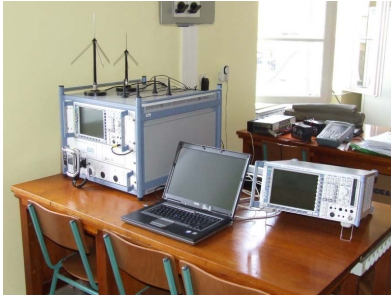
Slika 5.1. Radio Network Analyzer Rohde&Schwarz TSMQ (R&S ® TSMQ) mrežni skener
