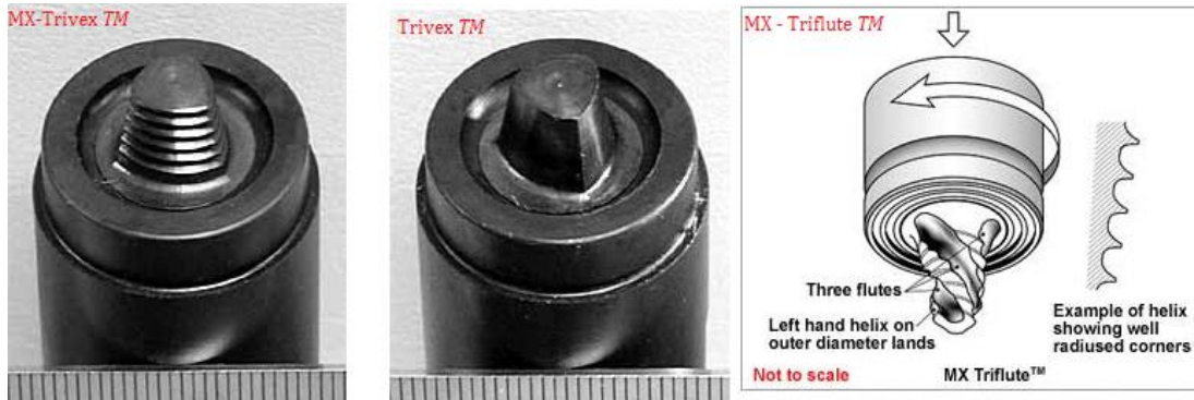
Figure 3.4 Examples of the MX-Triflute™ (right), TriVex™ (middle) and MX-Trivex™ (left) friction Stir welding tools.
