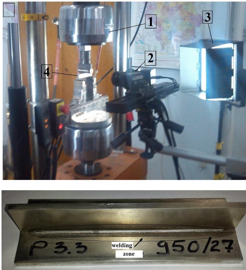
Figure 6.1 The experimental setup: 1) Test machine, 2) Cameras, 3) Light source, 4) Specimen
