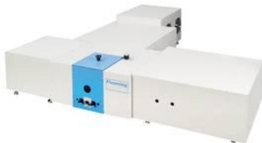
Slika 3.2. Fluorog-3 spektrofluorimetra ( Jobin Yvon Horiba, Paris, France)
