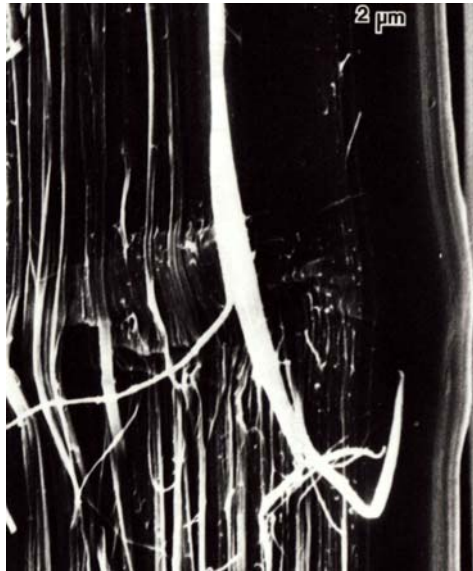
Figure 5-3 SEM micrograph revealing fibrillar microstructure in an as-spun PBZT fiber 127
