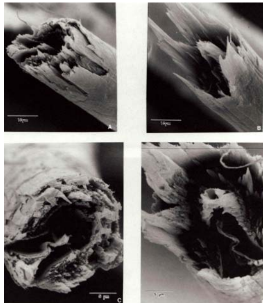
Figure 5-4 SEM side views (A,B) and endon views (C,D) of matching fracture ends of a tensile-fractured PBZT fiber. 127
