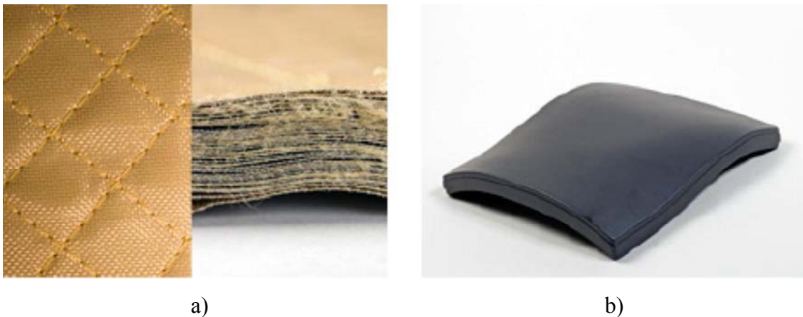
Figure 2-5 a) Fabric as example for soft ballistic b) protective plate as example for hard ballistic
