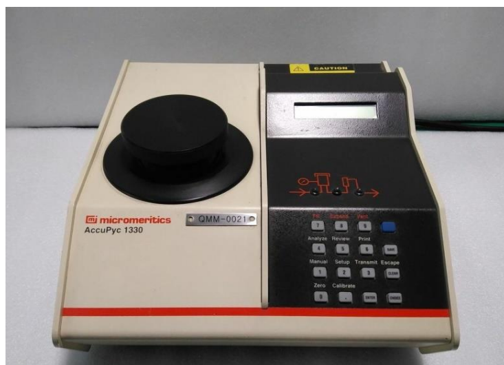
Slika 5.1: Automatizovani piknometar AccuPyc 1330 ( www.spwindustrial.com )
