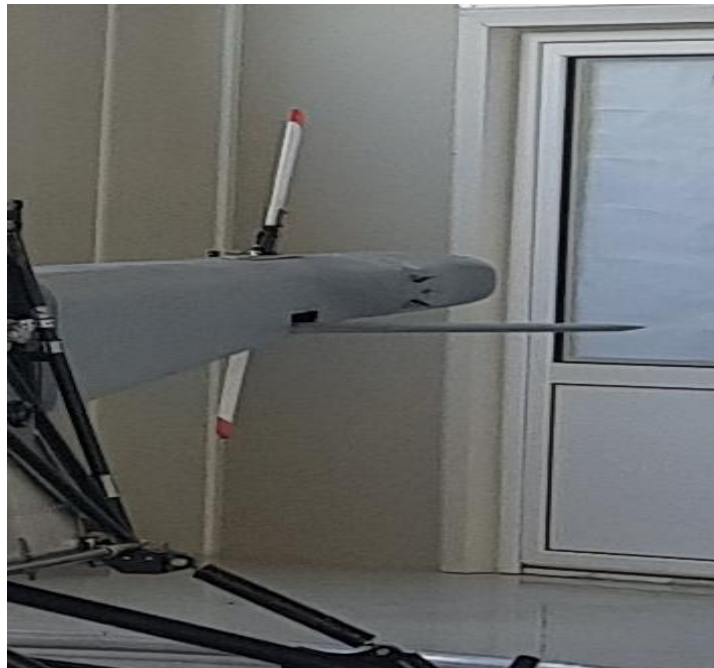
Figure 6.10: The final assembled Tail boom body
