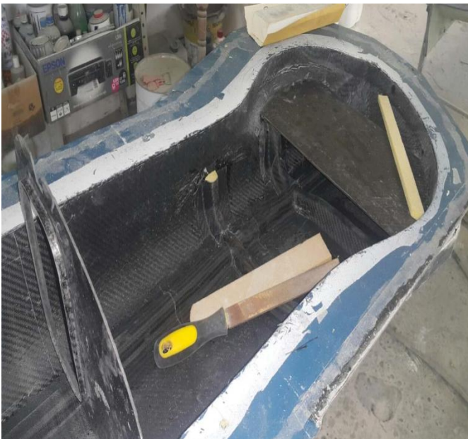
Figure 6.6: Placement of the Tail boom structural parts
