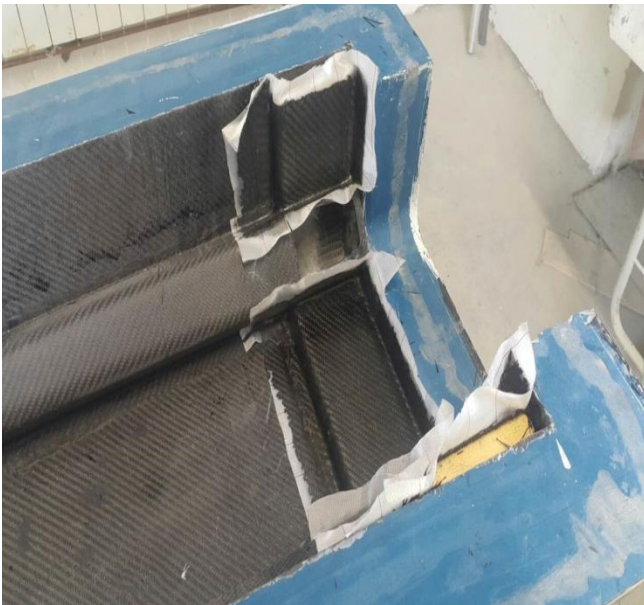
Figure 6.3: Hand lay-up of the carbon fiber composite material
