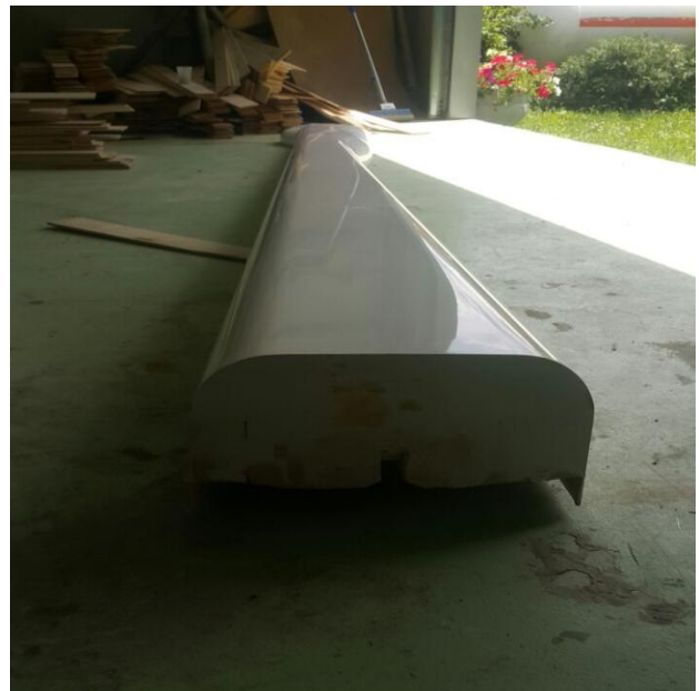
Figure 6.7: Outer shape of the Tail boom upper half
