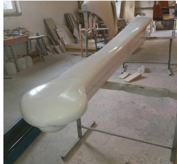
Figure 6.9: The Tail boom structure assembly
