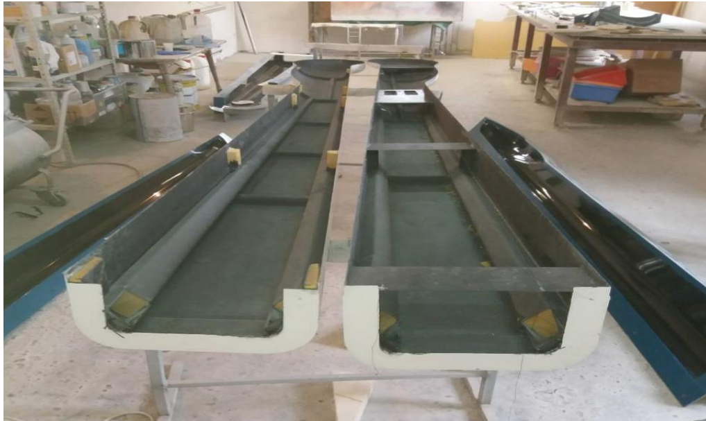
Figure 6.5: Manufacturing the upper and lower parts of the structure
