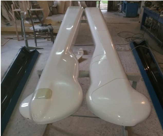
Figure 6.8: The outer shape of the Tail boom two halves
