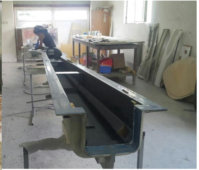
Figure 6.2: Hand lay-up of the Tail boom structure
