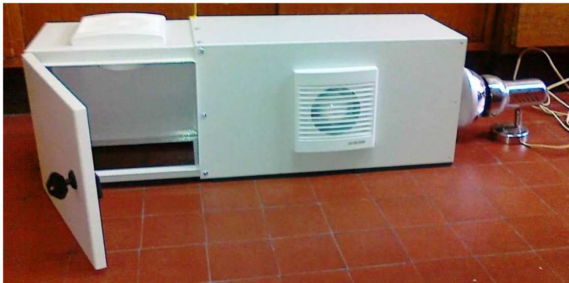
Figure 3.1. Photographs of the dark chamber and light sources used in the photoelectrochemical experiments.
